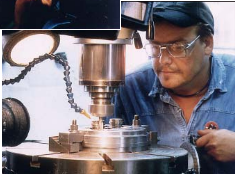
Manufacturing of dies (SAPA, Sweden).
