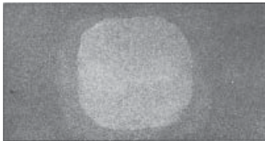
Uddeholm Impax Supreme welded with a dissimilar filler rod.
